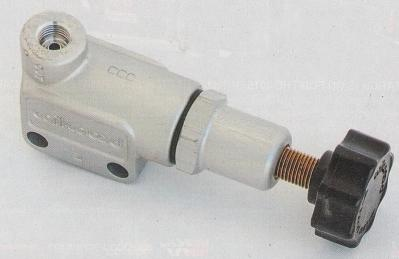
[Wilwood's knob-style adjustable proportioning valve lets you fine-tune the front to rear braking balance by proportionally decreasing the rear brake-line pressure. It weighs only 5.2 ounces and has two ¼-inch mounting holes spaced 1-inch apart. Shown is PN 260-10922 with 3/e-24 threads for SAE 3/16-inch inverted-flare tube nuts. Mount it anywhere in the line going to the rear brakes.
